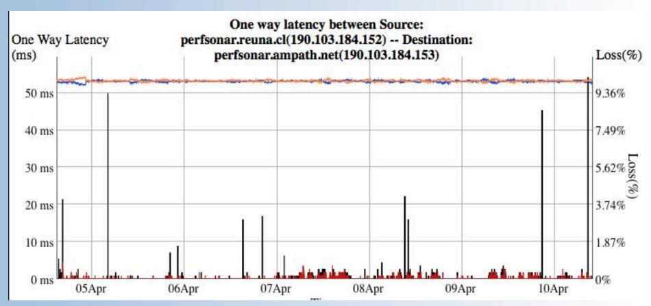
The Left Column shows the one-way latency with the orange the the blue lines (representing directions)
